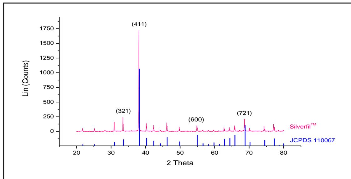
**Figure 1:** XRD diffraction pattern of Silverfil™ amalgam
