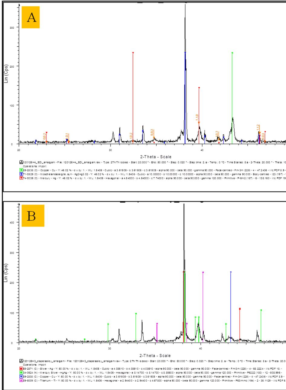
**Figure 2:** XRD pattern of two commercial amalgams; A. GS80 and B. Dispersalloy
