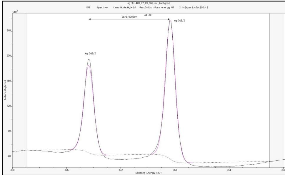
**Figure 4:** The narrow scan XPS spectra of Silverfil™
