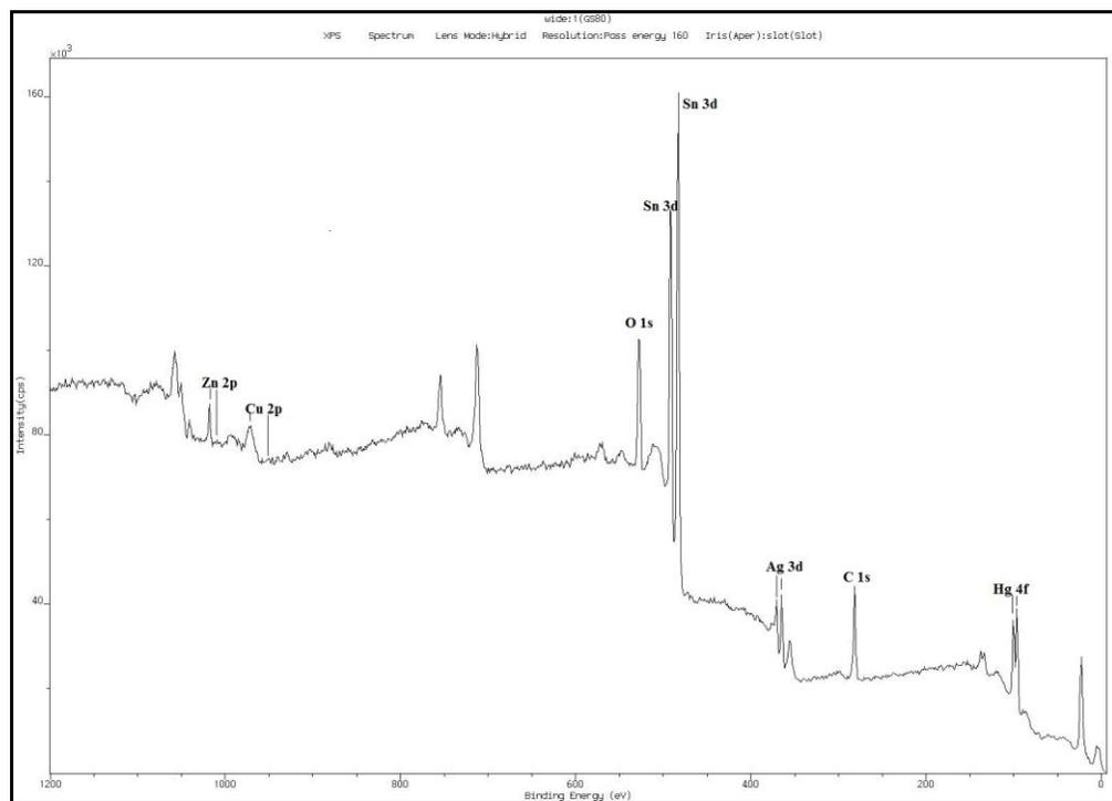
**Figure 6:** The wide scan XPS spectra of GS80
