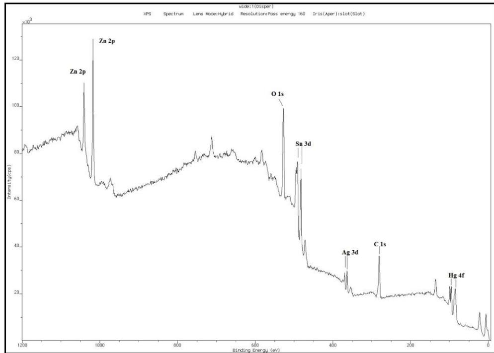
**Figure 7:** The wide scan XPS spectra of Dispersalloy
