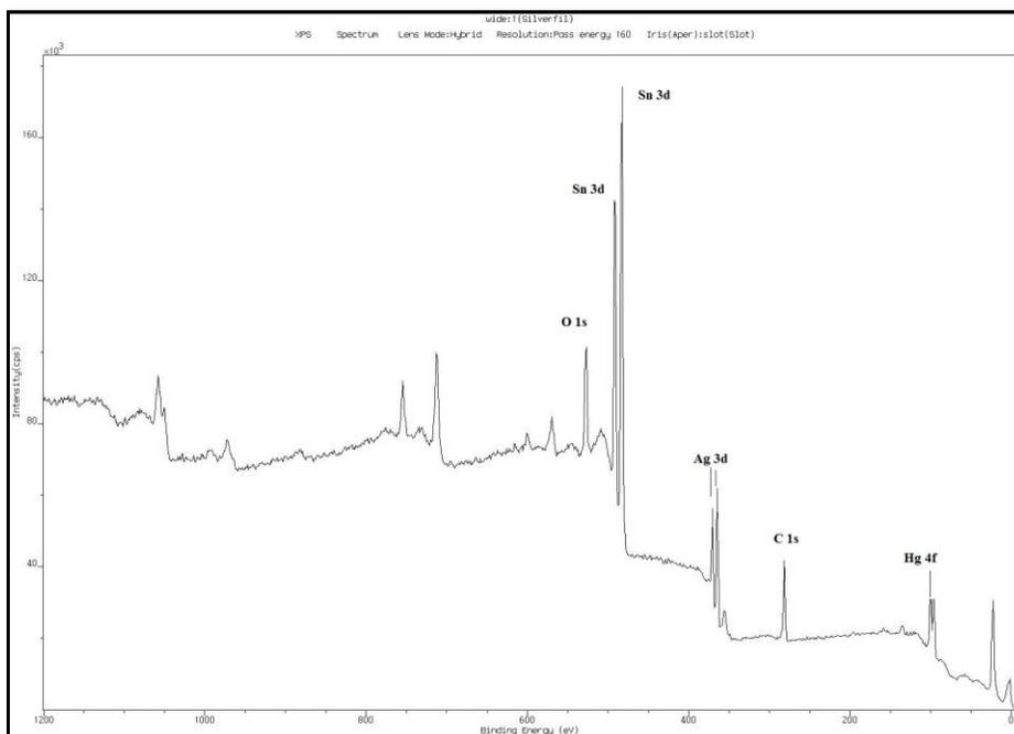
**Figure 3:** The wide scan XPS spectra of Silverfil™
