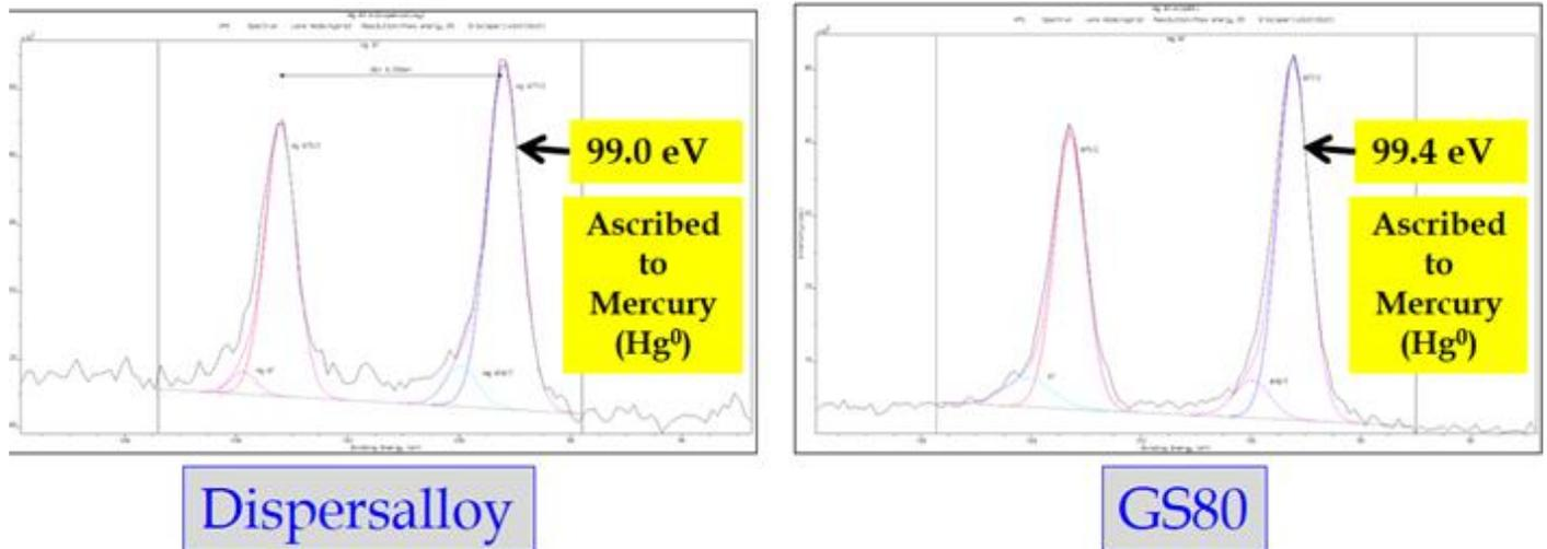
**Figure 8: The narrow scan XPS spectra of Dispersalloy and GS 80**
